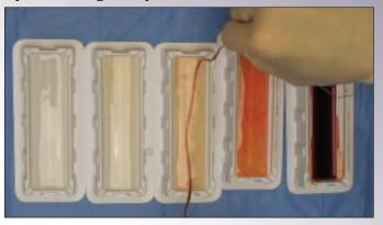
A Collagen Coated FiberTape and a standard FiberTape were used in a cadaveric SpeedBridge repair. This test proved that the collagen remains intact throughout a procedure. Both of these FiberTapes were dipped in a collagen dye prior to testing.
