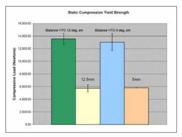
Figure 4. Static Compressive Yield Strength
