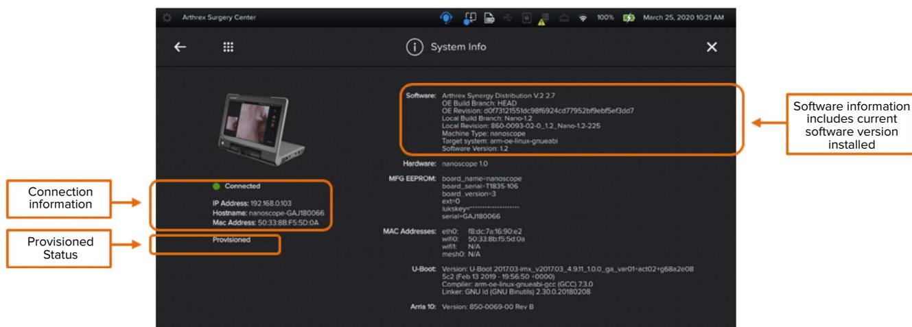
**Note:** If your device does not display active provisioned status, as above, please contact Arthrex Service. Device provisioning is required for remote support, remote software upgrades, and remote license activation.
