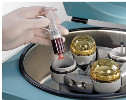
Centrifuge for 5 minutes at 1500 rpm.
