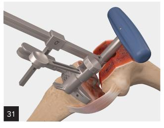
Set the depth of resection using the Tibial Stylus, dialing in the desired amount of resection (0 mm-10 mm).
