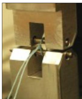
**Knot Security Test Set-up**
